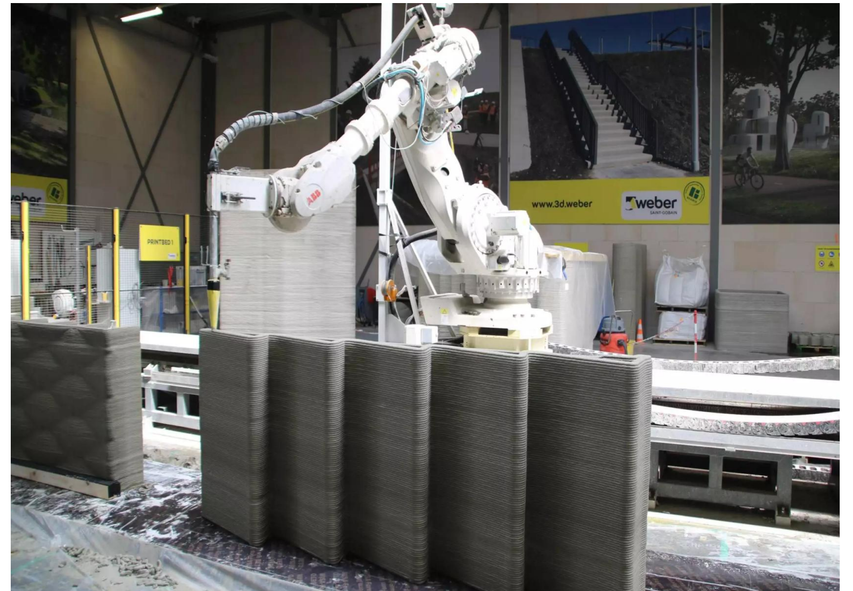
図3. Weber Beamix社の実機3DCP
